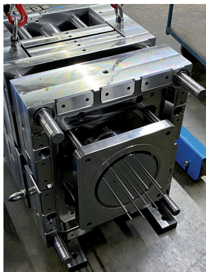
4/ Moving half of the mould with stripper plate
